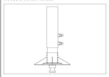
We have utilized a king pin that is suitable for the size and weight of the trailer.
