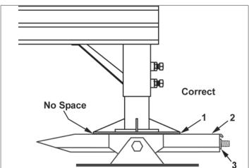
The king pin plate (1) must be in contact with the fifth wheel (2) with no space.
